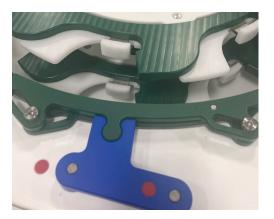
Simply take out the keys, expand or contract the guides and starwheels, and replace with the correct keys for the new bottle
